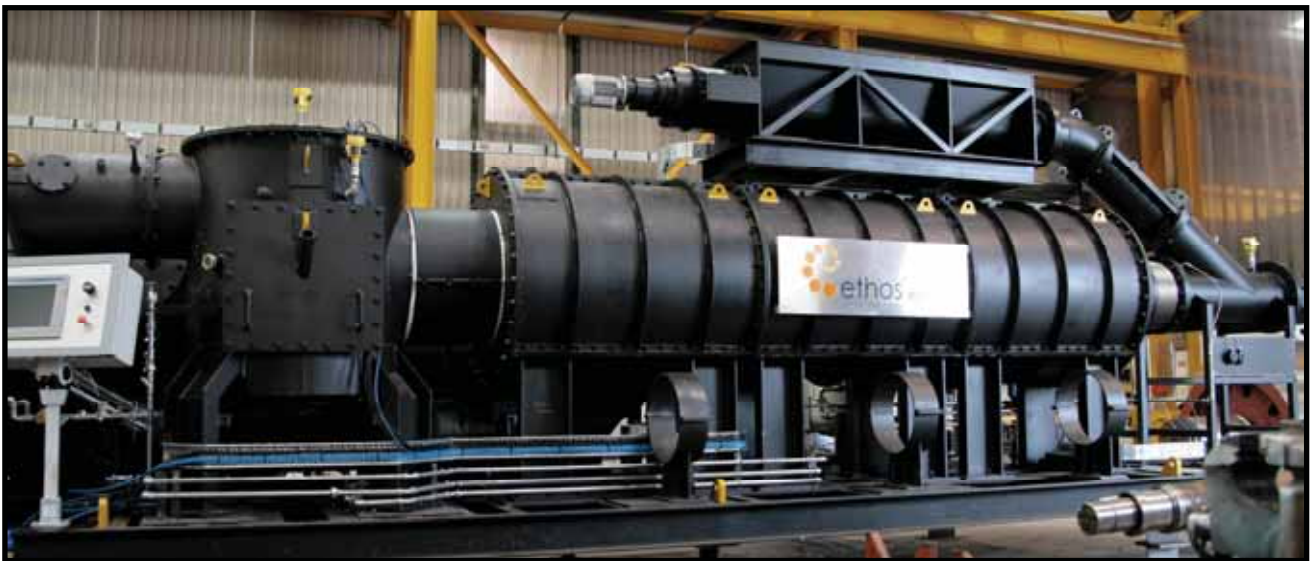
Ethos Energy's ST150, one of four being built for Queen Elizabeth aircraft carriers
